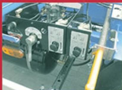
*On the dashboard you can find the controls for parking, lift axles and the 5-way valve.*
