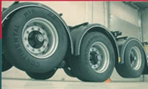
*As a standard option, the Flexitraler® can be fitted with a lift axle on its front axle. If desired, you can also have the rearmost axle fitted out as a lift axle.*
