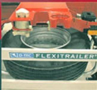
*A maintenance-free, hot-galvanized spare wheel carrier (excluding the spare wheel) is part of the standard configuration.*
