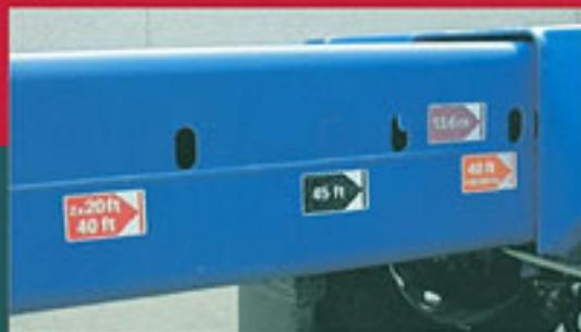
*The instruction stickers provide an easy-to-understand illustration of which extension positions go with which container types.*
