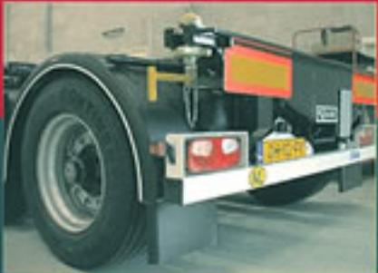
*To transport high cube containers, D-TEC also supplies the Flexitraler® with 385/55 R22.5 tires. This lowers the loading floor height from 1170 mm to 1100 mm without affecting the payload capacity. The tubular bumper shown is optionally available.*
