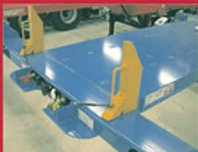
*Container stops help guide the container and protect the front bar, improving the lifespan of the trailer.*
